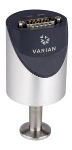
The Varian CDG-500 series of temperature compensated Capacitance Diaphragm gauges provides a high level of accuracy in the high pressure region. Full scale measurement ranges are available from 1000 Torr to 1 Torr. The CDG-500 series uses a corrosion resistant ultra pure alumina ceramic diaphragm providing exceptional signal stability, fast recovery from atmosphere, short warm-up times and unparalleled robustness.
