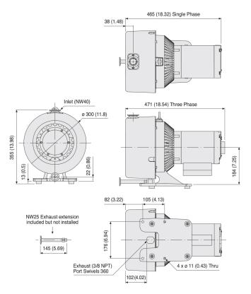
The TriScroll series is a range of two-stage dry scroll pumps that have high pumping speeds and low base pressure. TriScroll pumps eliminate the frequent maintenance requirements of oil-sealed rotary vane pumps, simplifying regulatory and environmental compliance, and eliminating oil disposal costs.
